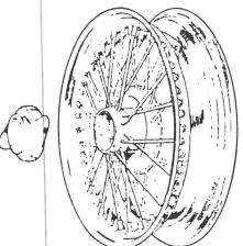
Knock it off: Twin Cam knock-offs (squared wing ends and flat lices) are NOT interchangeable with other knock-offs with the same thread. The inside tapers are different, and will damage your wheels. John Twist (AMGBA) **W** 130
