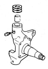
(from question on page 2) No, it's not a kind of fish. It's a fitting between two shafts which are at right angles to each other (#4 above). They are commonly found at the upper end of a king pin front suspension.
